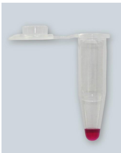
4. After shaking on vortex ColoredTaq mixes with the tube contents and is ready to work
